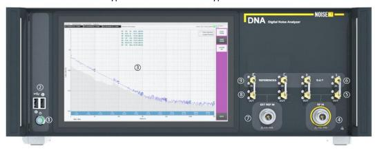
Figure 3 - DNA L (Lite) Front Panel View
